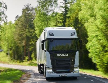
Tractor (4X2) 40t GCW, 330kW E-Motor
